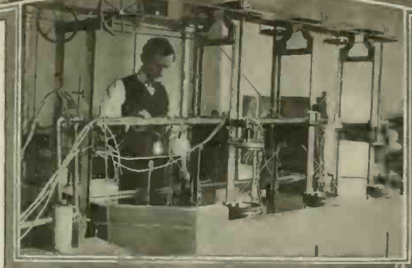
Photo © International Film Service These Men, Experts at the U. S. Bureau of Mines, Do Nothing But Play With Coal. The Calorimeters Above Are Used to Gage the Heat Value of Coal in B. T. U.
