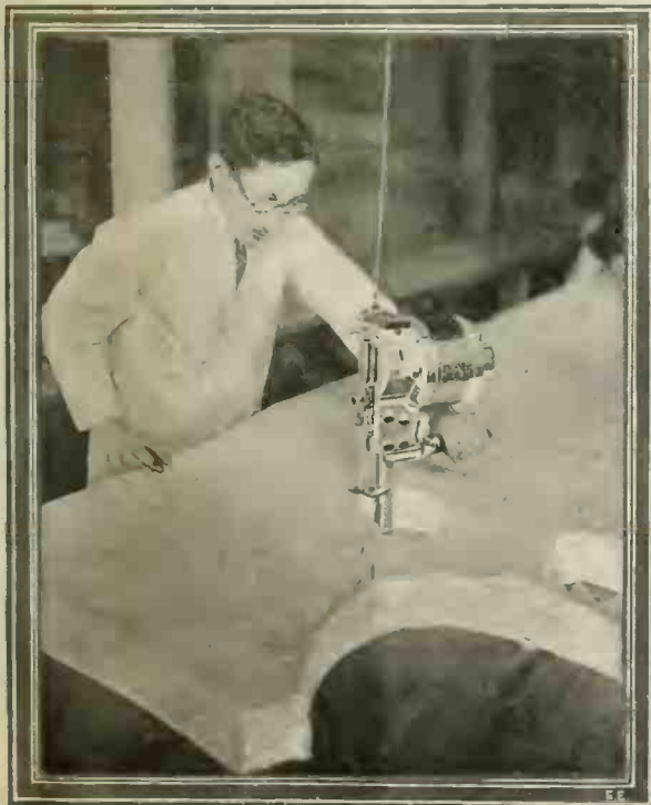
The Cutting Division of the Red Cross Does Its Work by Electrical Machinery. After the Pattern of the Garment Is Stencilled Many Thicknesses of Cloth Are Cut at Once with Motor-Driven Cutters of the Type Here Shown.
