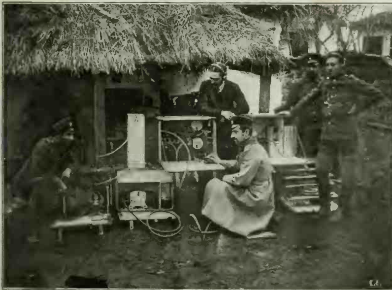
Photo © by International Film Service Portable Radio Set Used by the Bulgarian Army. It Can Be Carried on Mules Over Mountain Passes.
