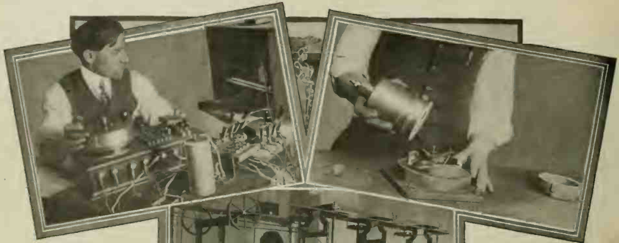
This Photo Shows Sample of Coal In Metallic Capsule, With Igniting Fuse and Bomb Calorimeter. Note Small Amount of Coal Used In Test.
