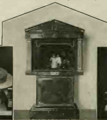
At Last—a Real Practical Show-Window "Movie" Machine. It Can be Set In Any Show-Window and Works Entirely Automatically. It Is Operated by an Electric Motor. It Uses Non-Inflammable Films Up to 500 Feet in Length. The Lamp Used is a 250 Watt Incandescent Type. It Rewinds the Film Automatically. Center Photo Shows "Movie" as it Appears to the Sidewalk Audience.
